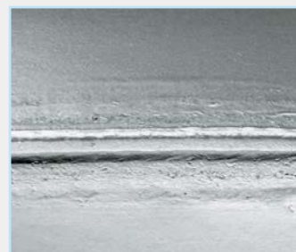
Above: Close-up of section of plasma welded pipe seam.
